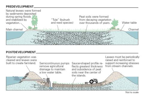
Figure 4: Diagram showing pre- and post-development of the Delta. Copied without permission from Ingebritsen, et al., 2000.
