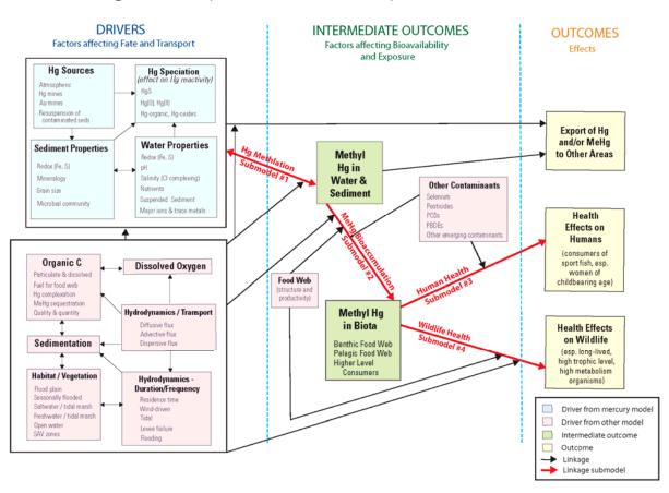
**Figure 2.** Mercury conceptual model showing four submodels. Drivers from other models (pink boxes) and drivers specific to mercury (blue boxes) represent important factors affecting the fate and transport of mercury. The formation of methylmercury in water and sediment (Submodel 1) is an intermediate outcome that leads to the bioaccumulation of methylmercury (Submodel 2). Methylmercury exposure can lead to adverse health effects in humans (Submodel 3) and wildlife (Submodel 4).
