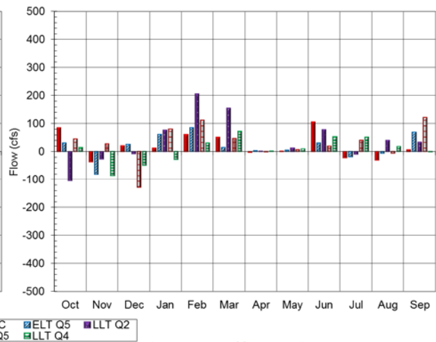
Figure 6-33: Changes in Exports at Jones Pumping Plant (Strategy 6 with and without Climate Change)
