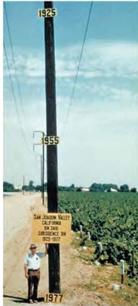
Figure 35: Excessive use of groundwater over time has led to groundwater basin depletion and substantial subsidence of land. This 1977 photo shows how many feet the land subsided as a result of groundwater withdrawal in the San Joaquin Valley from 1925 to 1977.
