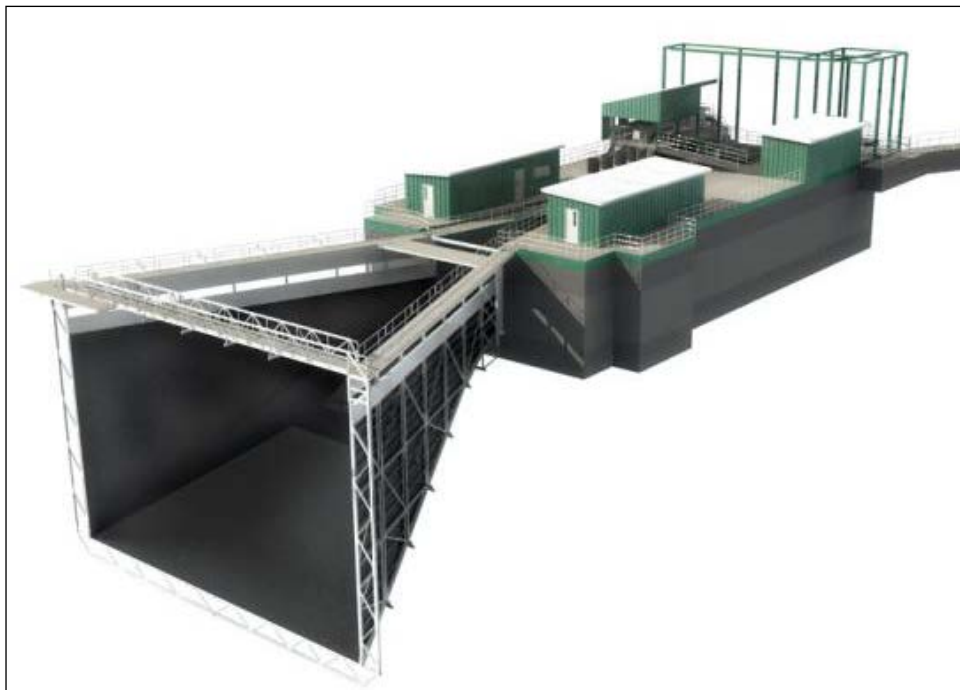
Figure 70: Isometric view of Upper Baker FSC and net transition structure (Courtesy of PSE)
