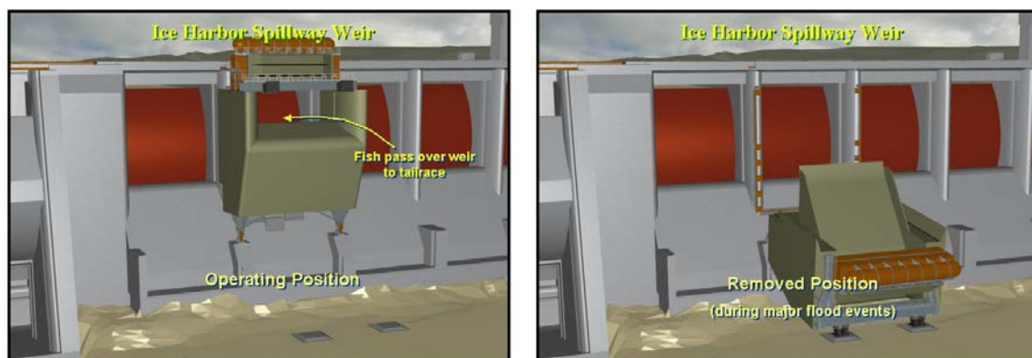
Figure 38: RSW in operating and non-operating positions (USACE 2011)
