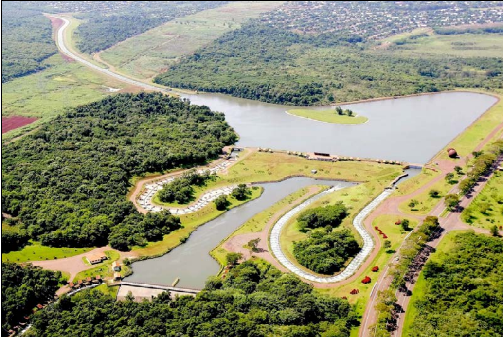
Figure 214. Aerial view of a section of the Canal da Piracema, including pond and fish ladders (Courtesy of Itaipu Binacional)
