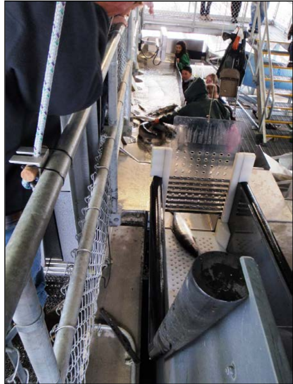
Figure 92: Cowlitz Salmon Hatchery – Fish being moved from shock box to upper sorting table (CA Dept. of Water Resources)
