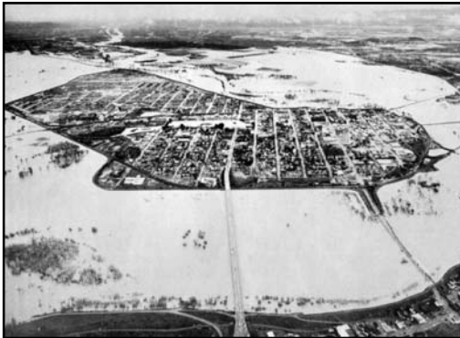
Source: California Disaster Office, 1956. The ring levee protects Marysville during the Flood of 1955
