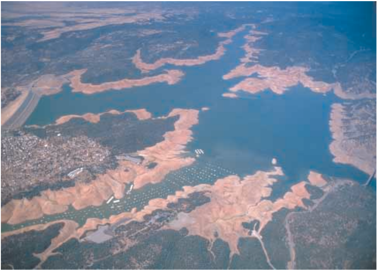
Lake Oroville in 1990. Oroville Dam is at left edge of photo. The 3.54 maf reservoir was at about one-third capacity at the time of this photo. During the 1976-77 drought, its storage declined to about one-quarter of full capacity.
