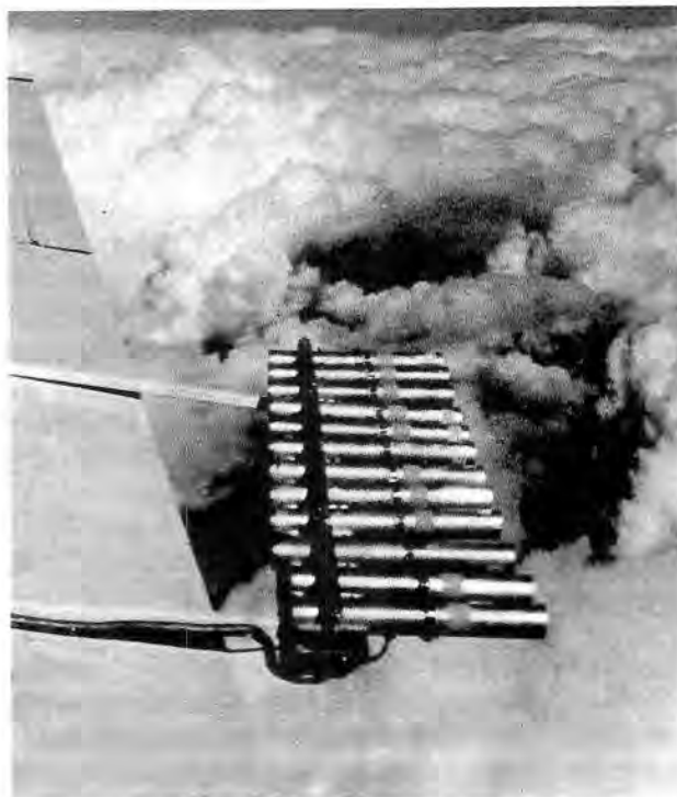
42. Cloud seeding by plane. Pyrotechnic seeding devices are shown while the seeding aircraft is in flight. Silver iodide nuclei are dispensed to produce rainfall more efficiently than if the clouds were left unseeded.
