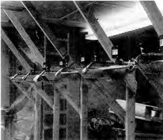
45. Which showerhead saves most? Numerous showerheads are shown being tested at DWR's laboratory facilities in Bryte, California. DWR tested hundreds of water conservation devices including toilet dams, flow restrictors, showerheads, and toilet bottles. (Note: The water was recycled.)
