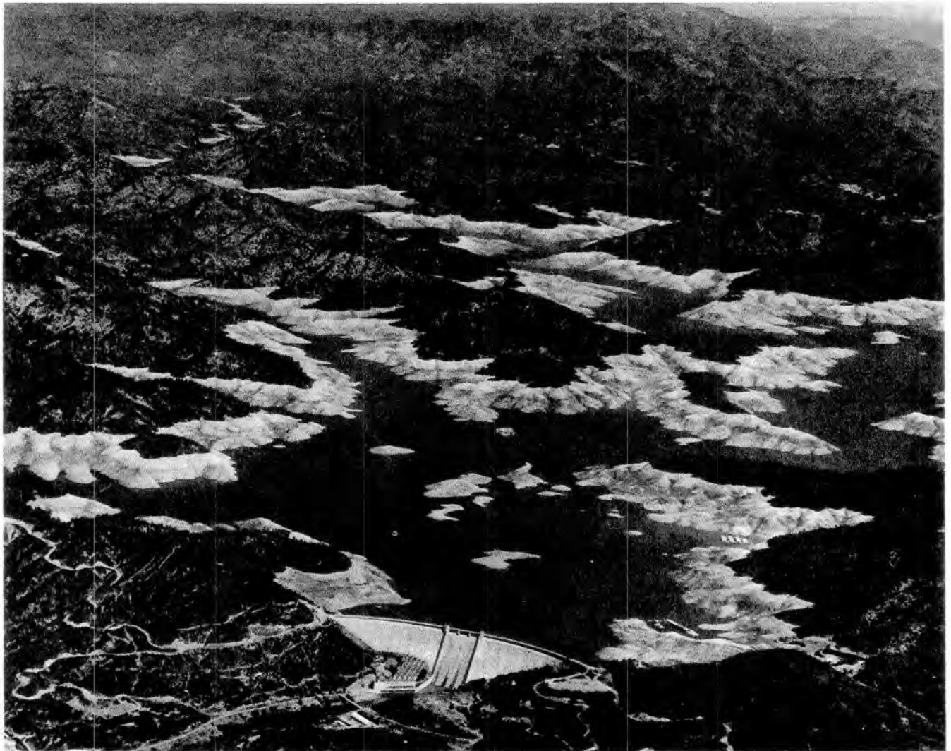
2. Low point for California's largest. Lake Shasta, formed at the junction of the McCloud, Pit, and Sacramento Rivers, is the primary facility of the federal Central Valley Project. This aerial photograph was taken on September 30, 1977, when the storage was 780 cubic hectometres (631,000 acre-feet), or only 20 percent of capacity. The low point was reached on September 14, 1977, with only 690 cubic hectometres (563,000 acre-feet).
