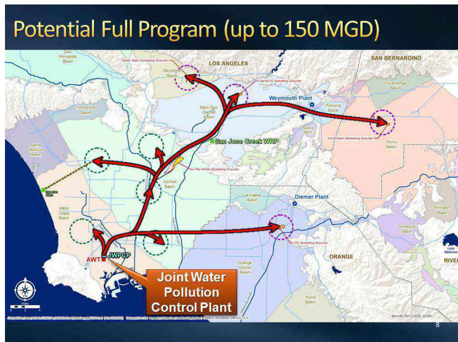
The Metropolitan Water District of Southern California’s plan with the Los Angeles County Sanitation District to treat water at the Joint Water Pollution Control Plant in Carson and replenish up to nine groundwater basins in the Los Angeles area.
