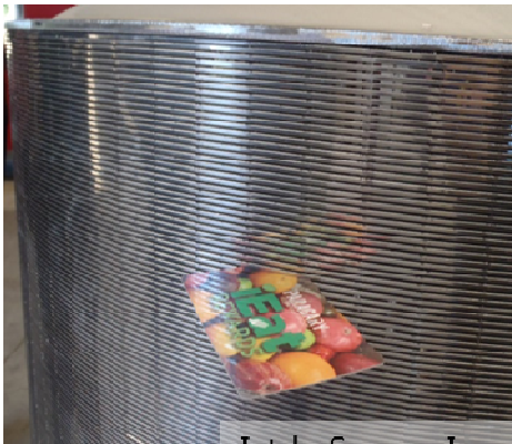
An example of a 1mm intake screen. These screens will be necessary for ocean water intake systems if subsurface intakes are infeasible in order to reduce mortality of fish and their eggs.
